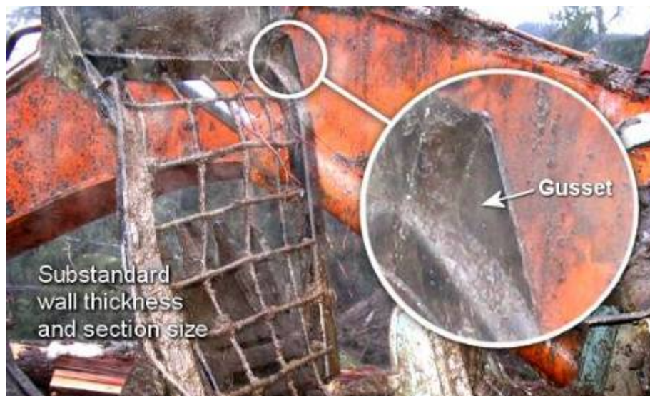
Photo 3: The operator protective structures did not meet requirements.
