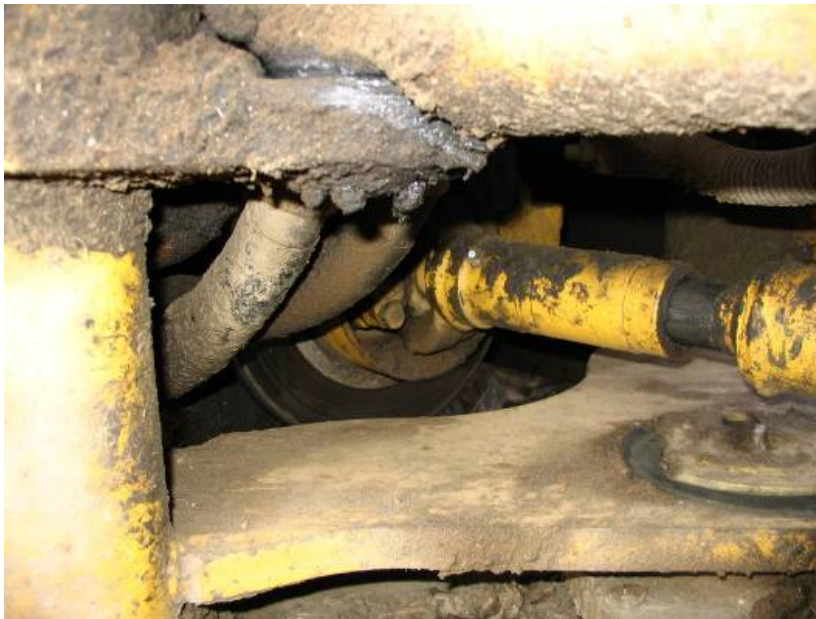
Photo 4: Transmission output coupling and driveshaft disc brake
