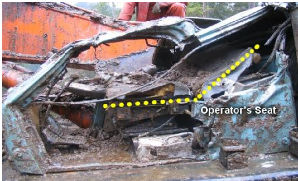
Photo 4: The crushed cab.
