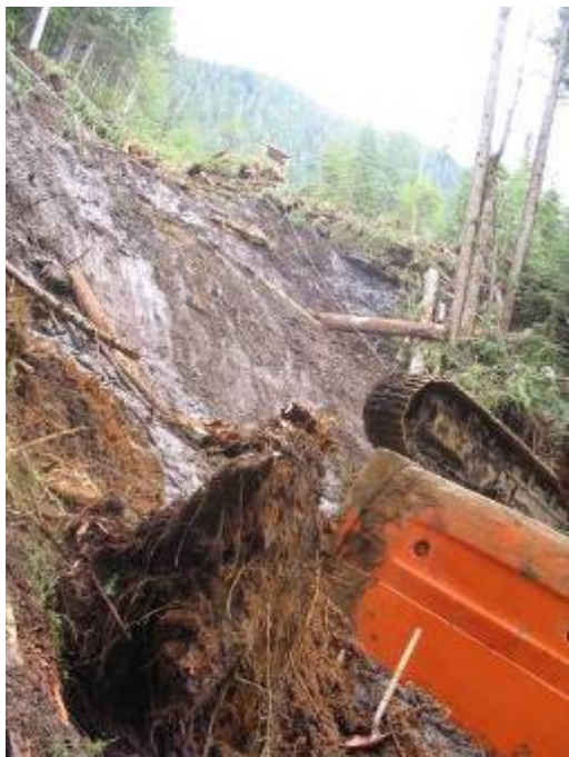
Photo 2: The excavator slid down a steep muddy slope and over a bluff.
