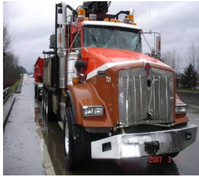
Figure 20: Damaged front end of Vehicle 3.
