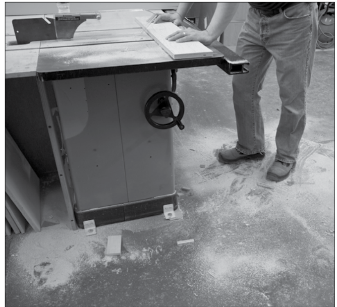
Sawdust accumulation around the infeed area of a power saw can create a slipping hazard.
