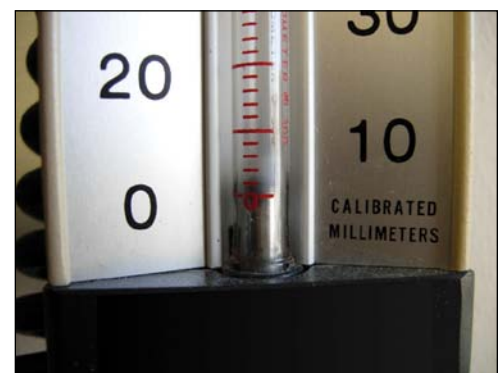
Mercury reservoir in a sphygmomanometer
