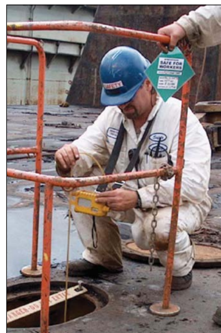
Worker testing a confined space on a barge
